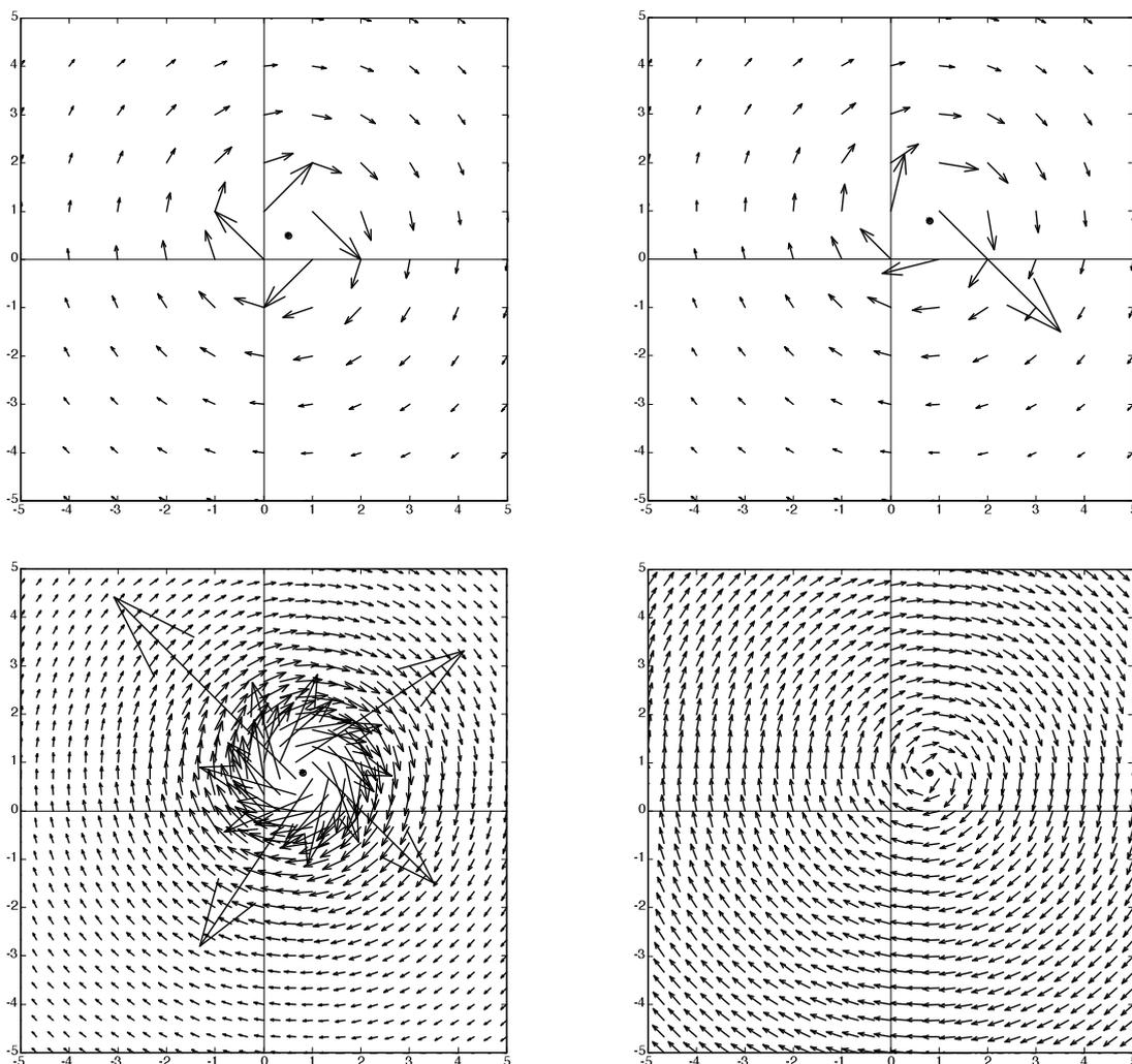
**Fig. 4.23:** Field strength vectors around a current carrying conductor.
