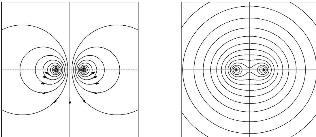
**Fig. 4.26:** Current carrying two-wire conductor. Field lines with direction arrows (left), contour lines of equal field strength (right). Lines of equal field strength are not equipotential lines ( $\rightarrow$  Fig. 4.27).
