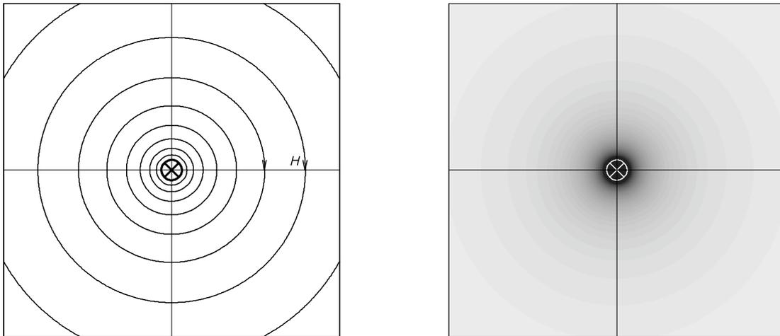
**Fig. 4.25:** The magnetic field of a current carrying conductor. Left: Field lines. Right: Gray tone coded. The gray tones produced by printers and copiers are not able to resolve the radial field decrease with sufficient precision.
