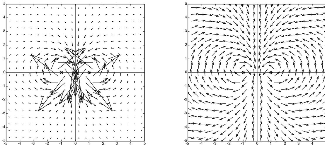
**Fig. 4.24:** Field strength vectors of a current carrying two-wire conductor (left) and the normalized version (right). In the right image, asymmetries between the upper and the lower part of the picture can be perceived, again based on the misinterpretations shown in Fig 4.23.
