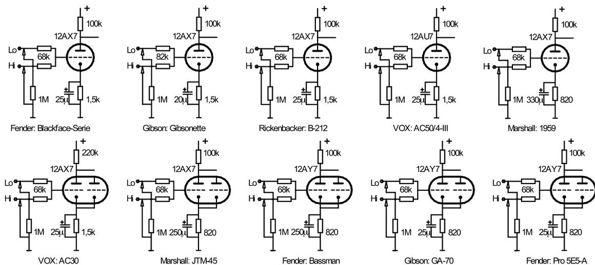
**Fig. 10.10.1:** Input circuits of various guitar amplifiers.
