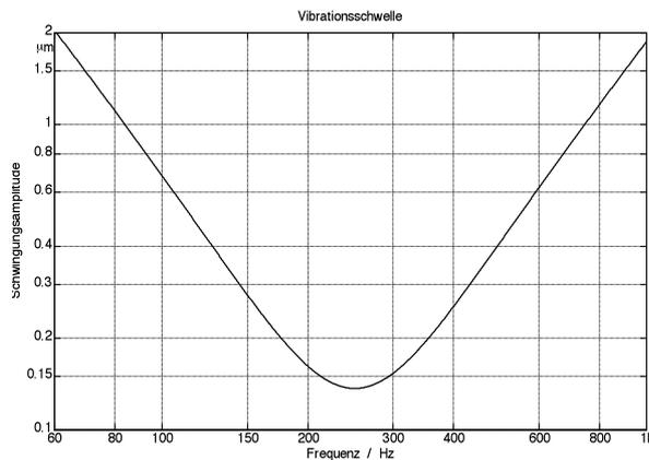
**Fig. 8.47:** Vibration threshold. Only values above the threshold lead to a perception of vibration. According to this graph, a vibration of an amplitude of 0,4  $\mu\text{m}$  can be felt at 300 Hz; at 800 Hz it would not be felt anymore. “Schwingungsamplitude” = vibration amplitude; “Vibrationsschwelle” = vibration threshold
